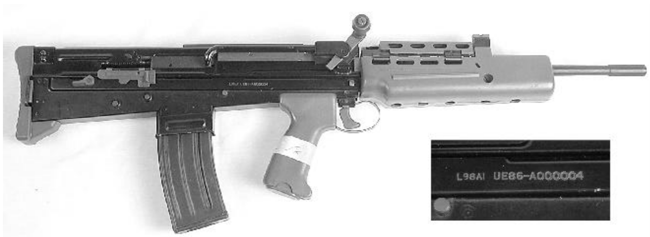
L98A1 Cadet rifle, single shot version of the SA80 for Cadet training. There is no gas system, this is entirely manually operated. There is a 22LR Subcaliber unit available for this unit.
