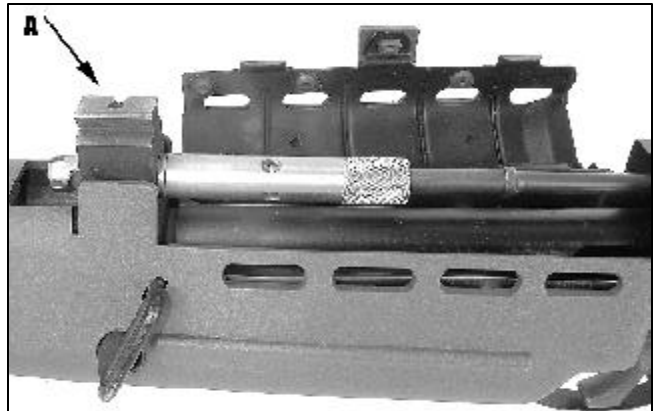
The gas piston system is exposed when the handguard upper is opened to the right. Note the post base for a fixed style front sight (A).
