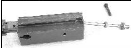
Disassembled bolt carrier assembly. Examine for cracks, chips, or any signs of wear.
