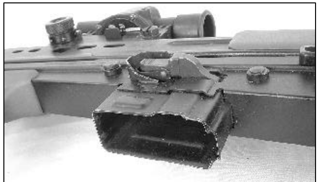
The magazine catch is protected from accidental pressure, which is a good thing, however, the thin sheet metal walls of the magazine well are prone to damage, and more importantly, the "Bell" of the well, where magazines enter, is prone to damage as well- making magazine insertion difficult or impossible.
