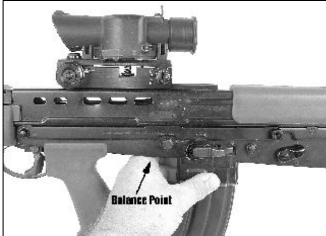
The Balance point is several inches behind the pistol grip. This leads to a tendency for the rifle to rotate downward when held in a standard style- balance is important to fully automatic firearms, not having a secure platform for the buttstock will lead to erratic shot placement. It is important to fire this weapon with a good, solid two hand hold, secured against the shoulder.
